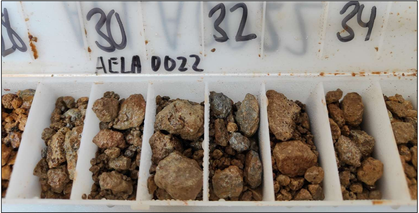
Figure 3: Nickel sulphide anomalism intersected in AELA0022 (4m @ 0.62% Ni, 310ppm Cu, 177ppb Pt+Pd from 32m) within saprock ultramafic with dark purple-red pits indicating weathered nickel sulphide mineralisation.
